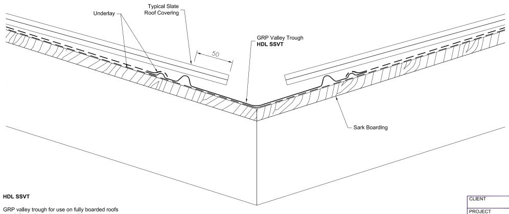
GRP valley trough for use on fully boarded roofs specially designed for the Scottish market. In standard lead grey colour.
